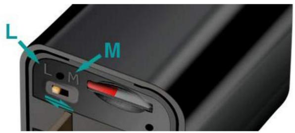
2. Motion detection mode: When Your Smart Charger is set to "M" position, and the device is plugged into the power supply, the blue LED indicator light will flash 3 times. In this case, the recorder is set
